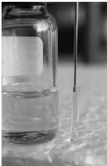
Fig. 7. SPME needle placed in 8 \mu\text{L} extraction vial with 3 \mu\text{L} acetone being present.
